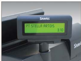
The SPS-500 Series has an adjustable Rear Customer Display.
